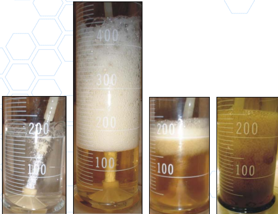
Figure 2 Amine solution foaming conditions (left to right); a) No foaming, b) surfactant caused chemical foaming, c) foam inhibition by antifoam, d) THE BEAST
